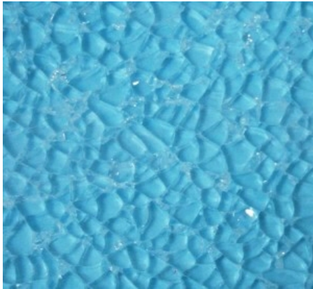
Close up photograph showing how toughened glass splashbacks shatter when broken
